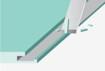
Use chisel or cutting tool to remove the locking portion of the floor, then apply the special adhesive. Install the floors together horizontally.
